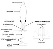
Figure 8. External view of mortar ammunition concept.
