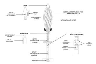
Figure 9. Internal view of mortar ammunition concept.
