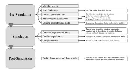
Figure 7. Simulation phase steps.
